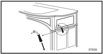
Fig. 16 Attach thermostat handle.
